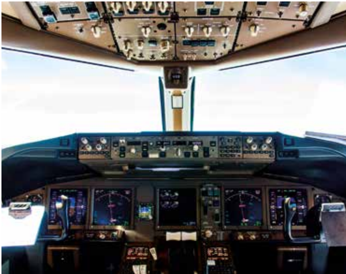
The flight controls of the Boeing 777 are operated via the fly-by-wire system.
