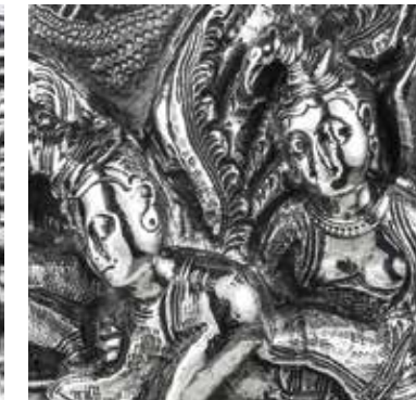
5.37 Early stage overpolishing – lost details on the face
