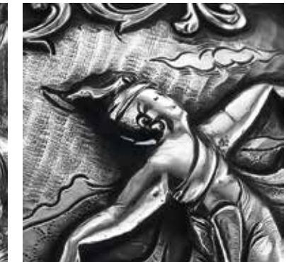
5.38 Late stage overpolishing – face is smooth without detail
